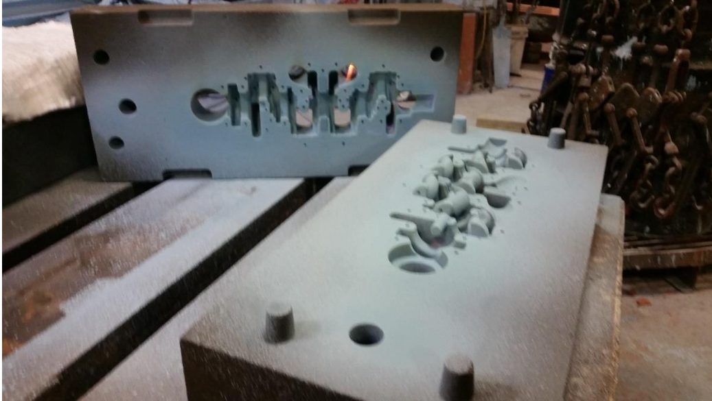
Figure 4.1 Cope and drag of one of the two sand molds used to cast the prototype steel crankshaft.
