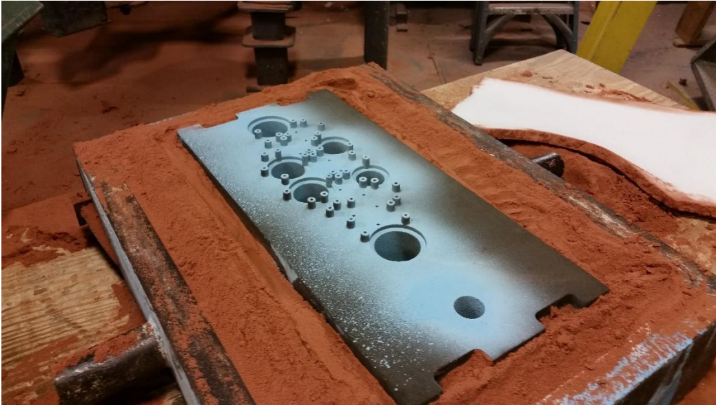
Figure 4.2 One of two molds, surrounded by packed sand in a flask, before filling.
